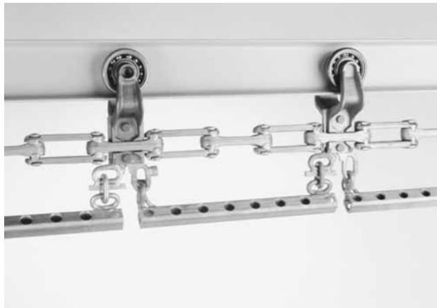
*Figure 7* – Continuous load bar: A more general purpose adaptation of the versions shown in Figures 4 and 5.
